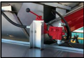
Hydraulic Control Valves
