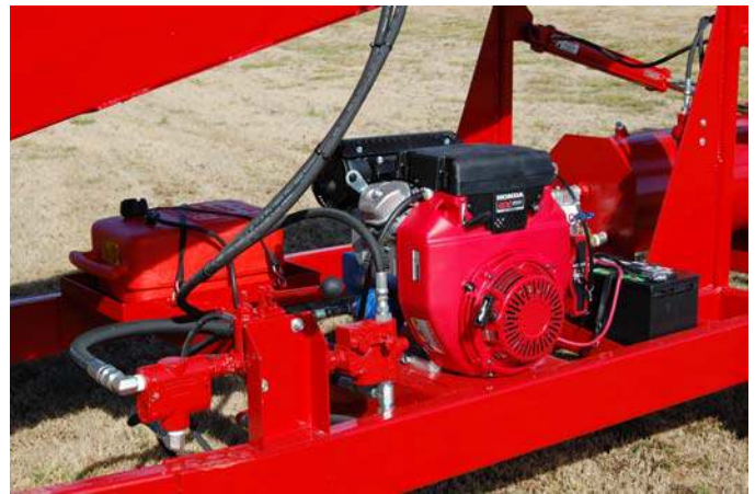
Self-Contained Hydraulic System
