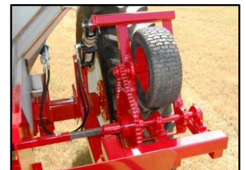
Press Wheel Drive Assembly w/ Cylinder Engagement
