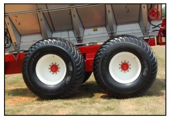
Tandem Axle Walking Beam Suspension:
