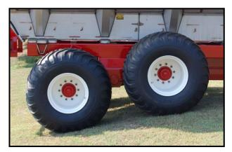
Tandem Axle Walking Beam Suspension:
