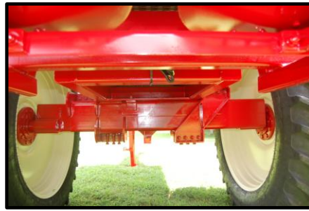
True Adjustable Track Axle
