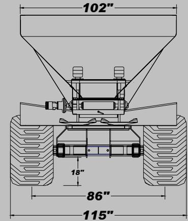
*All Products and Specifications subject to change without notice. Drawing shown with 45 - degree slope sides and Belt Over-Bar Type Chain.*
