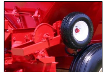
Press Wheel Drive Assembly with Cylinder Engagement
